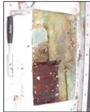
Wet deck repair: (clockwise, top left) Pilot holes drilled in deck to determine extent of wet core. The small area got larger with every drilled hole; Outer skin and core removed from area of core repair; Removing the wet core; New foam board in place with one layer of System Three resin.
